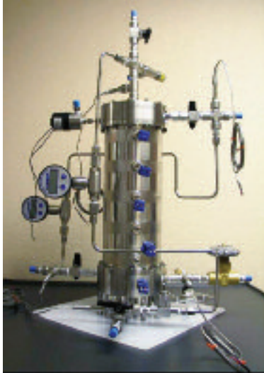
Hardware demonstrating full functionality of MTSA concept
