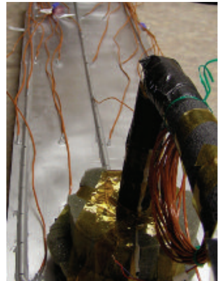
Stagnating radiator sub-scale test article
