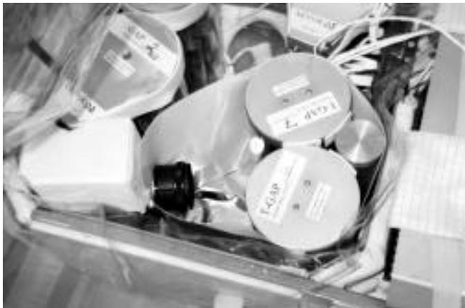
Figure 1 The small cylinder contains the light. The two larger cylinders marked T-GAP each contain an ABS. The video camera is shown at left.
